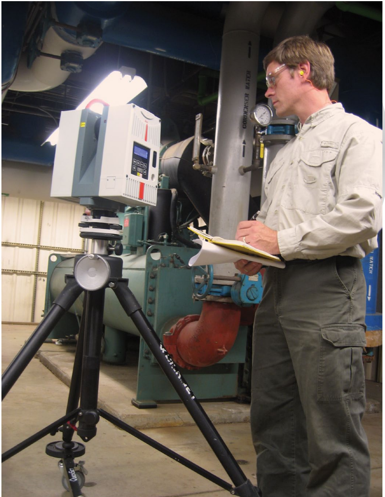
The right tool for the job... McKim & Creed utilizes high-speed phase-shift laser scanners for industrial and indoor projects. Survey party chief Dennis Batzel operates the scanner in the basement level of the Cates Boiler Plant.
